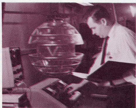
In orbit, the satellite will spin about 180 revolutions per minute, which will make it tend to remain pointed toward the same direction in space. But it must be well balanced so that it does not wobble or tumble. Dynamic spin balance test is shown.
