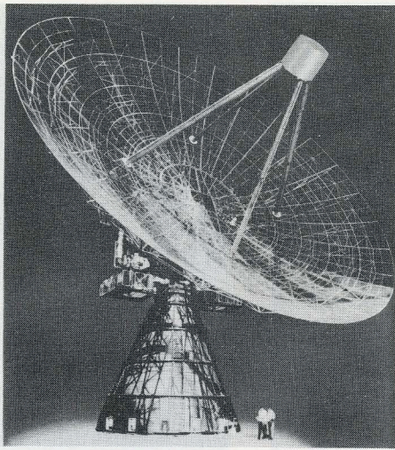
GIANT DISH — This tracking radar, 84 feet in diameter, is now in operation for testing purposes at RCA's Moorestown, N. J. plant. It is the prototype of tracking radars to be used in the third BMEWS site, at Yorkshire, England.
