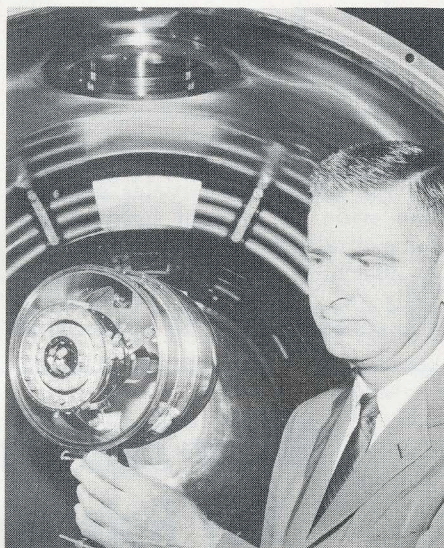
POWER TO THE PLANETS — An ion engine, demonstrated for the first time recently, is shown above. This type of propulsion, which could be the key to very long range space travel, generates less than a tenth of a pound of thrust by accelerating ionized cesium atoms.
