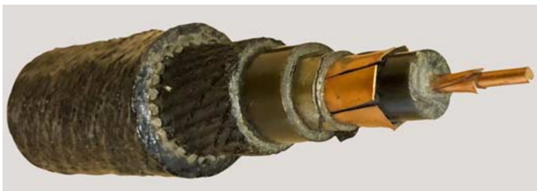
Section of the overland cable at the Clarenville Heritage Society museum, showing the additional components. Photograph by Jason Stringer
