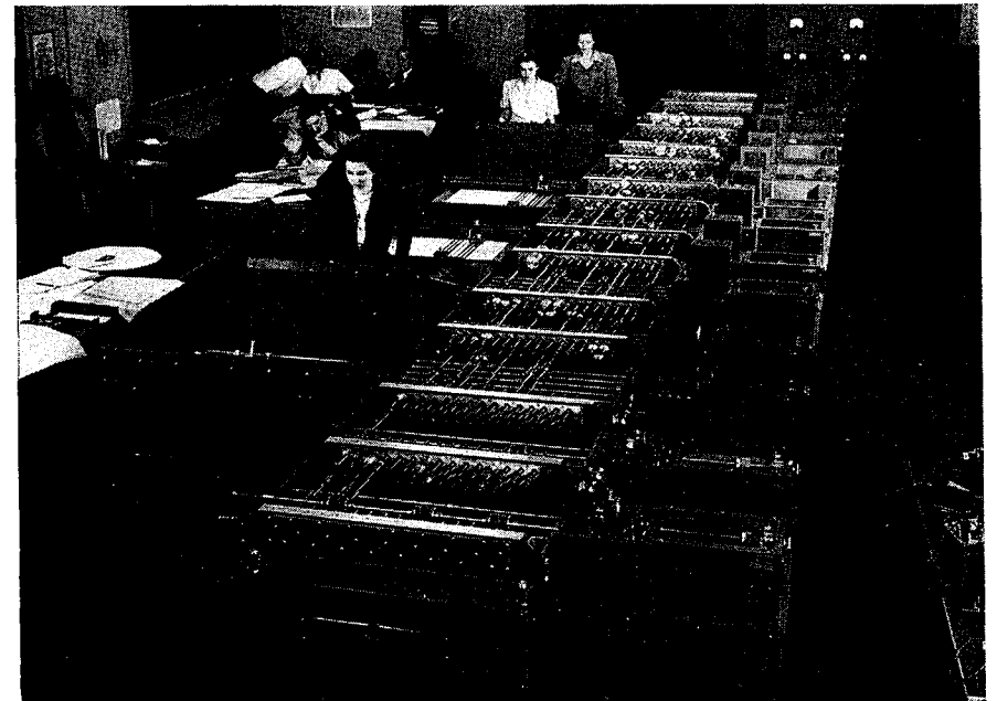
High-speed differential analyzer provides quick solution of complex mathematical problems.
