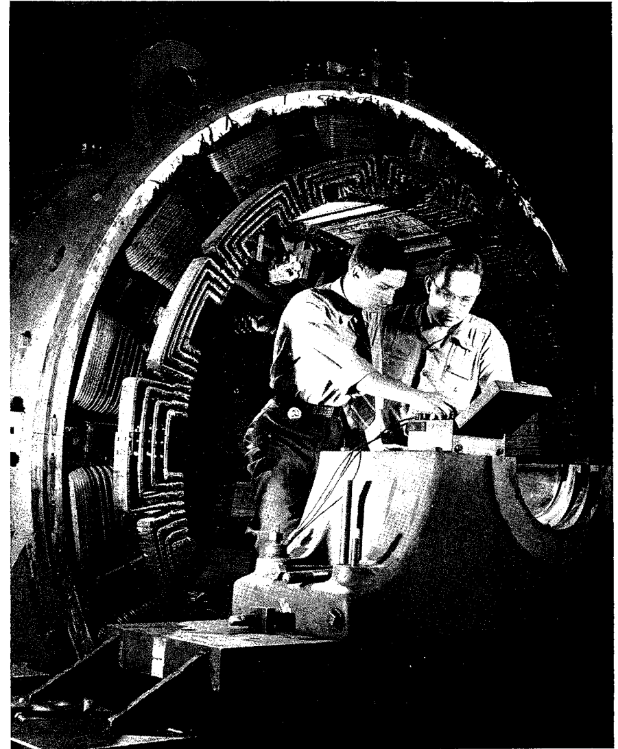
A test foreman checks an engineering graduate student in the test of a marine motor stator.
