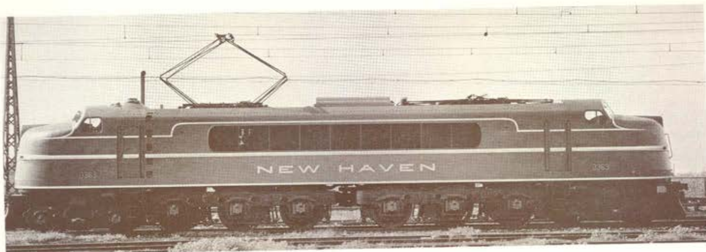
Streamlined High-speed Electric Passenger Locomotive, 3600 HP- Described in One of the Papers of the Transportation Session.
